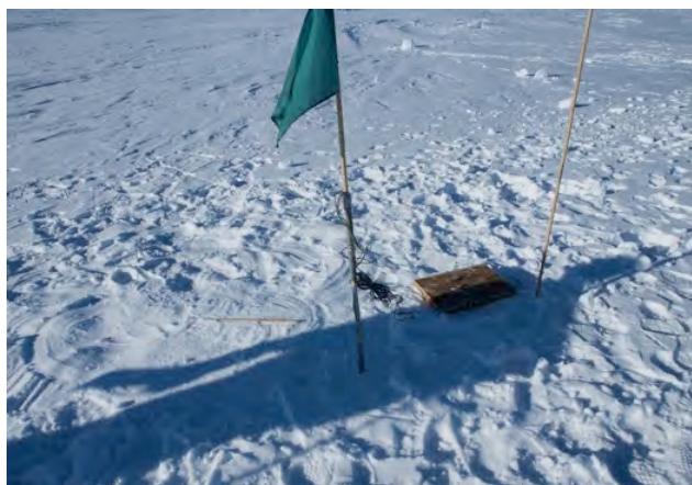
Fig 16. View of the thermistor set-up after installation is finished. Photo: John Fegyveresi.
