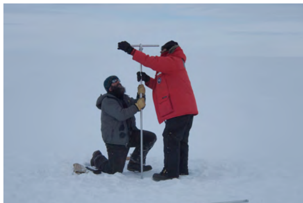
Fig 7. Jeremy Miner and Ross Beaudette drill a shallow ice core, WAIS Divide, Antarctica. Photo: Bradley Markle
