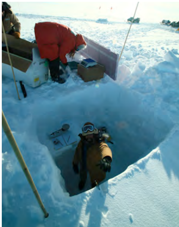
Fig 8. John Fegyveresi, Emily Longano, and Brad Markle sample a snow pit for stable isotopes and density measurements, WAIS Divide Antarctica. Photo: Graham Colegrave
