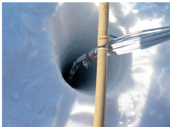
Fig 15. Installing the thermistor string. Photo: John Fegyveresi.
