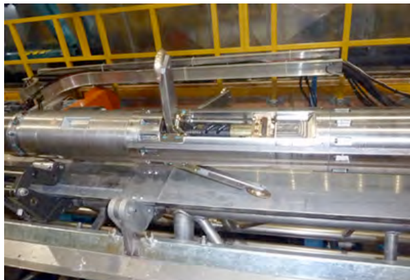
Fig 3. Replicate coring system actuator section. Photo: Chris Gibson, UW-Madison/IDDO.
