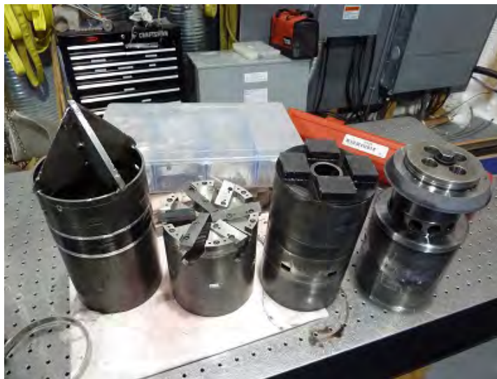
Conical Tool Used for Recovery of hardware, Milling Head, Magnetic Recovery Tool and Broaching Head
