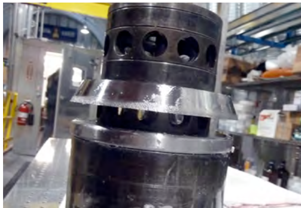
Fig 4. Replicate coring system broaching head. Photo: Chris Gibson, UW-Madison/IDDO.
