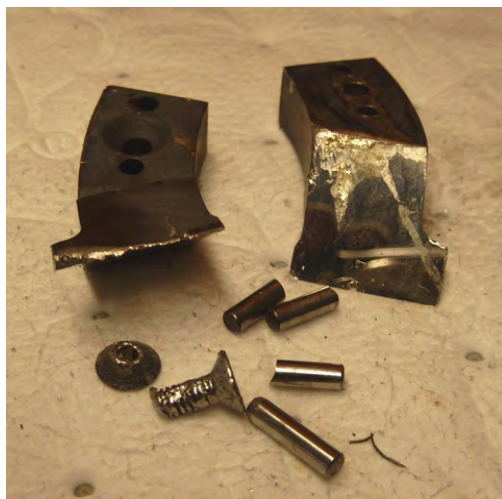
Broken Cutter Hardware Recovered from Deviation
