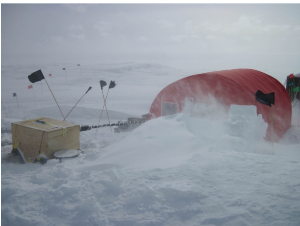
Fig. 1: Logging shelter located adjacent to the drilling arch. The logging cable exits the shelter, passes over a sheave wheel (inside a protective box), before dropping into the arch. With the shelter, logging operations were able to continue unimpeded through the poor weather that was prevalent during the 2011-12 field season.
