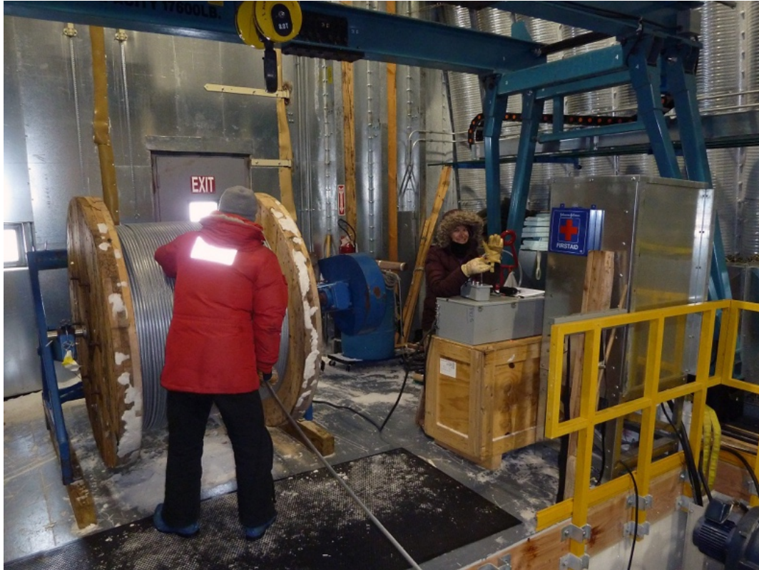
Unspooling of the old 3400-meter-long drill cable from the DISC Drill's winch drum. Photo: Kristina Slawny
