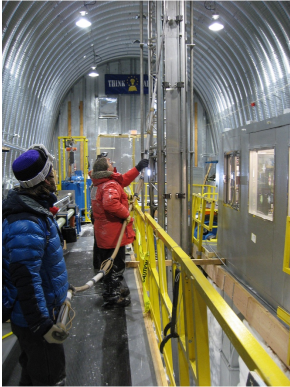
Figure 1. The five-meter-long sonic-logging tool is about to be lowered into the drill slot. In the foreground, Dan is holding the transmitter section. The flexible tan hose-like sections separate the transmitter and the receivers, and prevent propagation of sound waves directly through the tool itself.
