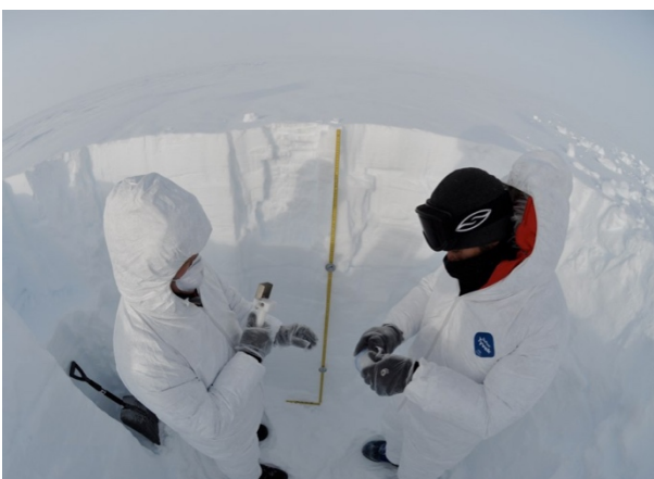
Fig 3. Gifford Wong and John Fegyveresi sample a snowpit for density, major ions, water isotopes, particulates, trace elements, and microbial loading. Photo: Logan Mitchell.
