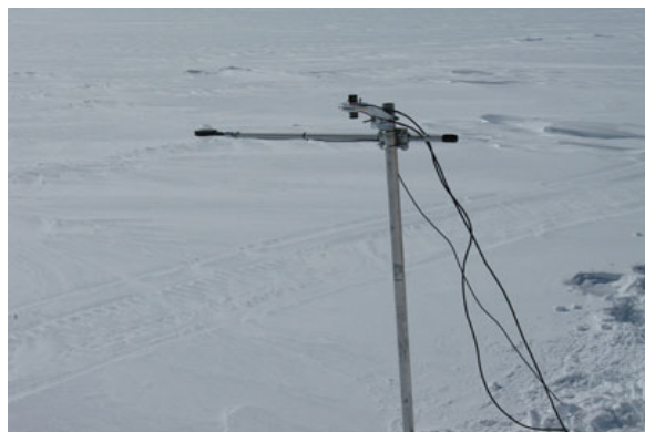
Fig. 1: Net radiometer and double-pyranometer setup. Photo: John Fegyveresi.
